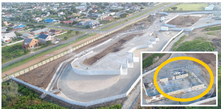
Materials-recovery and public drop-off facility currently under construction in Hermanus. The inset shows the location of the steel construction that caused the delay.
